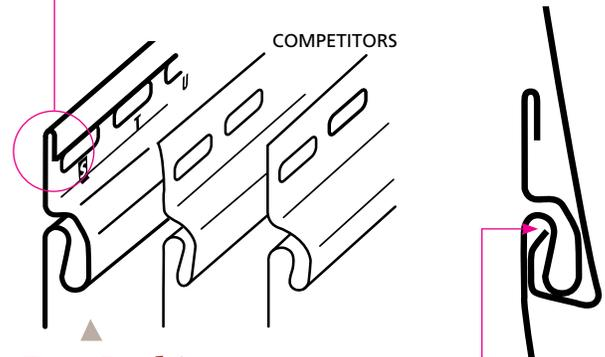
**DuraLock®** features an oversized rigid tear-drop shape which is substantially larger than many competitors' locks, providing secure installation.
